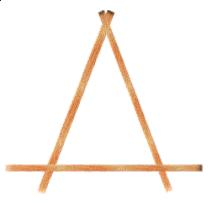
Lay out the 2.4m spars as shown in the diagram and lash the spars together with a square lashing where they cross.
