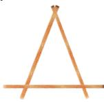
Lay out the 2.4m spars as shown in the diagram and lash the spars together with a square lashing where they cross.
